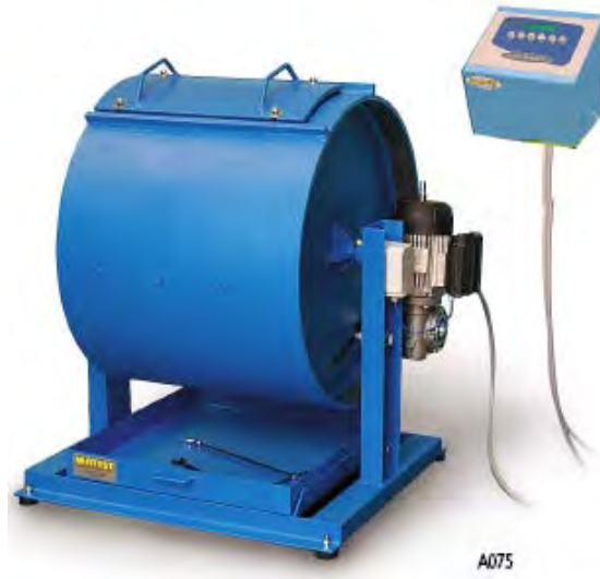
Figure 24: LA Abrasion machine (Qualitest International, Inc. 2009).
