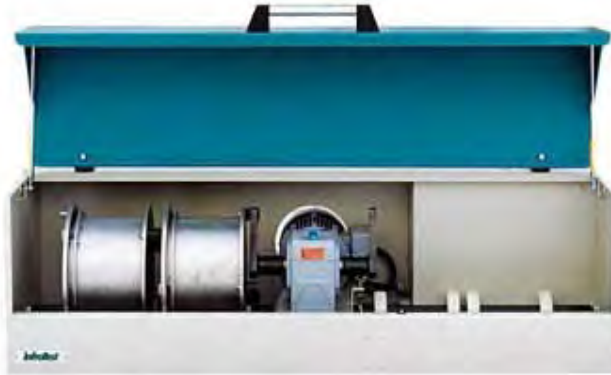
Figure 25: A Micro-Deval test machine (Inopave 2003).
